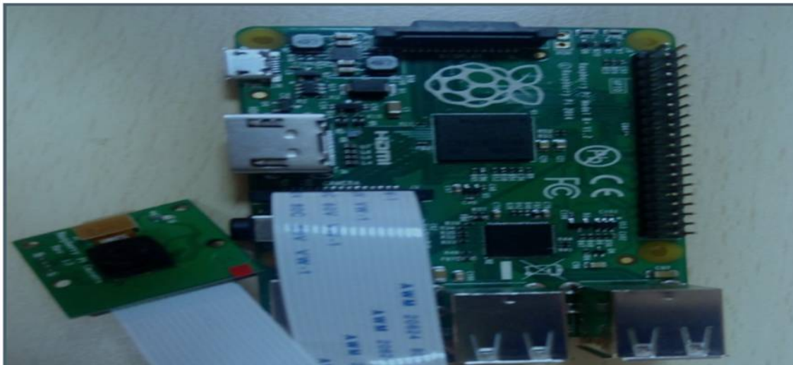
Figure 6 Interfacing of Raspberry Pi and Camera Module
